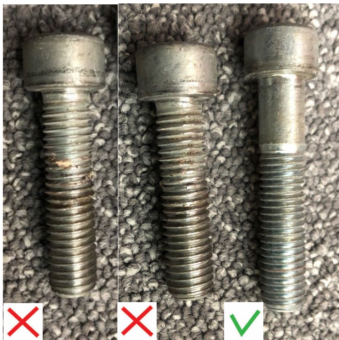
Picture 12. Use only not damaged M10 bolts.
